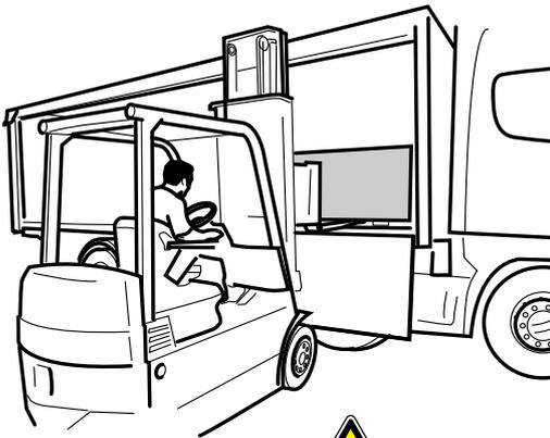
If the tiller is contained inside a wooden crate, use a fork-lift truck with suitable capacity to unload it (consult technical features table to see tiller weight) or use the lorry's lifting arm.
