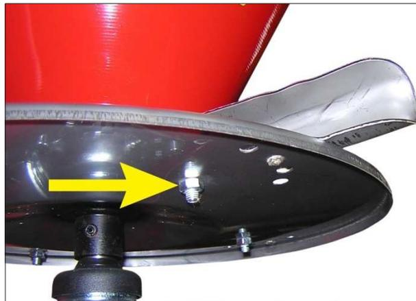
Unscrew the nut and replace the damaged vane.
