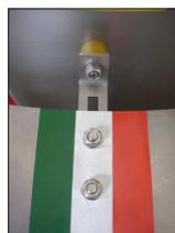
Now you can assemble the bracket (ref. 11 e 12) on the frame using the screws and bolts on it (pict. 3).
